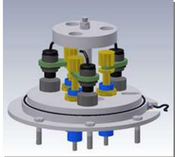
Long base extensometers are mainly used to monitor vertical or horizontal deformations occurring to many civil engineering projects such as embankments, foundations, dams, tunnels, diaphragm walls, instrumented piles, etc.
