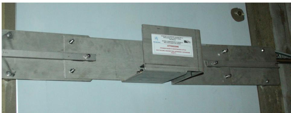
Specially developed joint-meter for the caissons of the MOSE project (safeguard of Venice)
