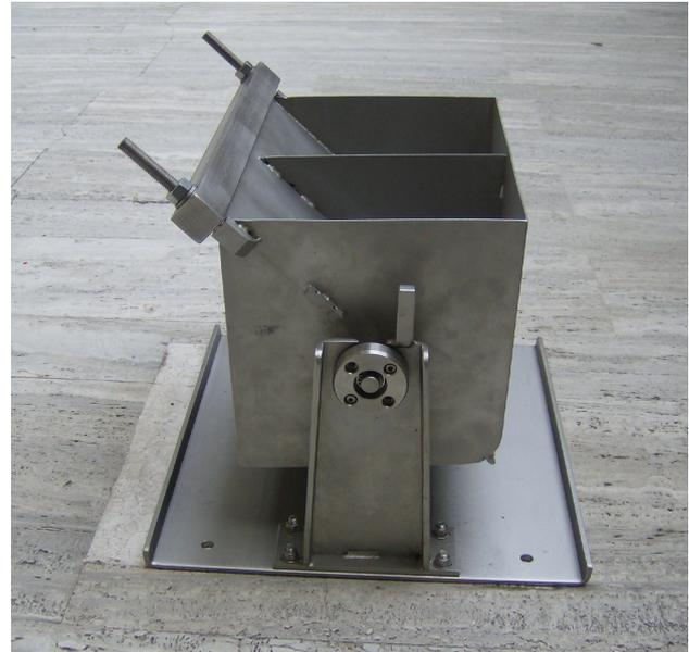
AGISCO's tilting bucket type flow gauges are very effective in measuring slow flowing open drainage channels.
