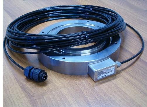
Load cells find wide applications in the field of civil engineering. They are mainly employed to measure and control tension in cable and rock anchors, on walls, diaphragms and structural beams.
