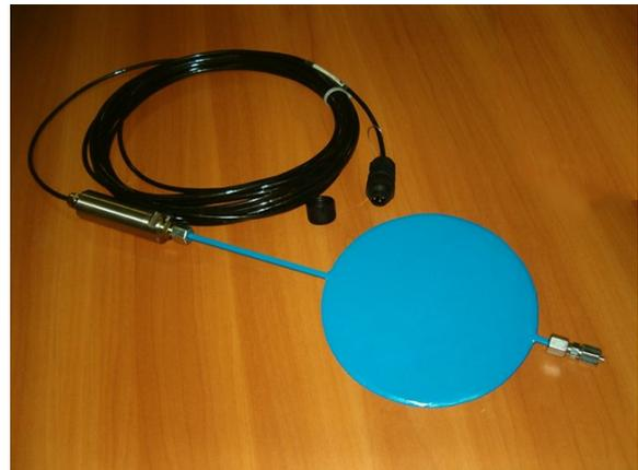
Hydraulic pressure cells were developed to measure the total load in embankments and foundations and are mainly used in dams, tunnels, bridges.
