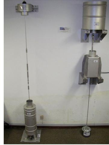
Pendulums are widely used in civil engineering to monitor rotation movements in structures. They are used in many types of construction such as dams, viaducts, buildings and in all cases where highly accurate long-base rotation measurements are needed.
