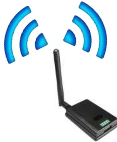
The new data transmission system developed by Agisco and based on the W-PAN (Wireless Personal Area Network) protocol reads and acquires different types of electrical signals such as current, voltage, strain-gauges, temperature, resistance, and many more.
