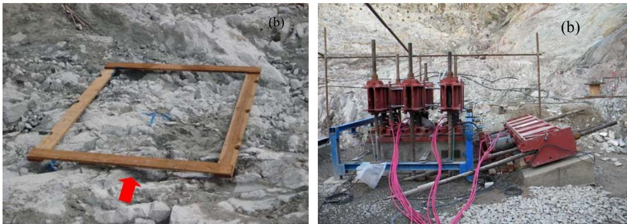
Figure 8: Testing site: (a) rock surface to be sheared, (b) photograph of the shear test apparatus
