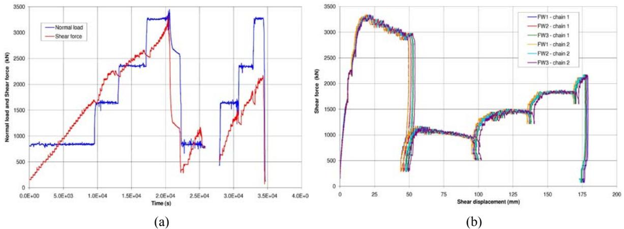
Figure 10: Results of direct shear test on concrete-rock interface with stepwise procedure
