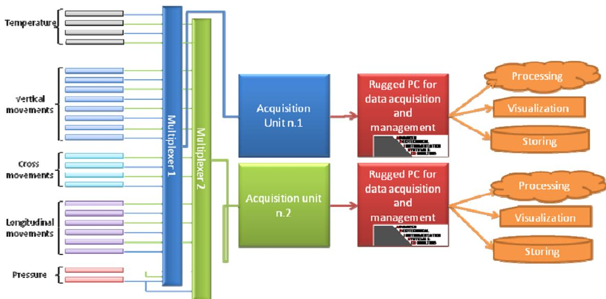
Figure 6: Layout of the data acquisition system
