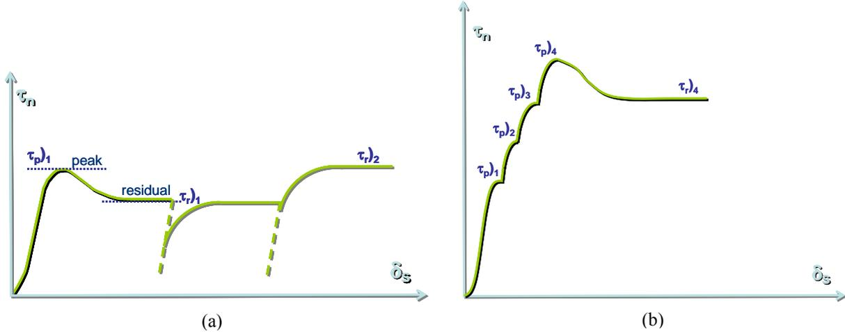
Figure 7: Schematic visualization of direct shear test
