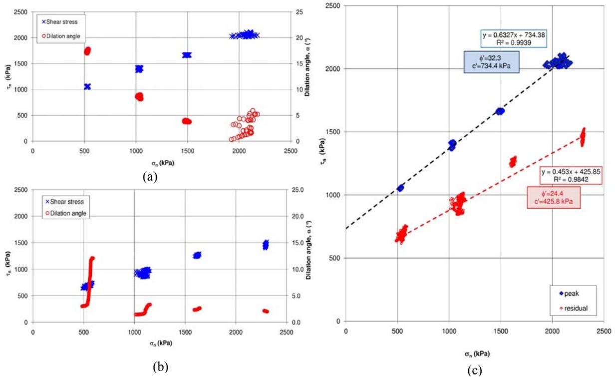
Figure 11: Results of direct shear test on concrete-rock interface with step-wise procedure
